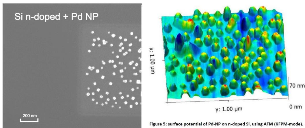
Figure 5: surface potential of Pd-NP on n-doped Si, using AFM (KFPM-mode).
