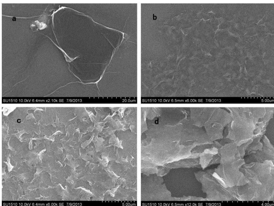
SEM images of (a) GO, (b) RGO\_NaBH<sub>4</sub>, (c) RGO\_MW, (d) RGO\_NaBH<sub>4</sub> + MW.
