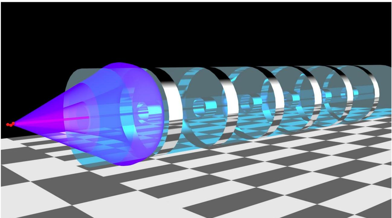
*Cherenkov light cone created by particles moving through a metamaterial designed by Chalmers researcher Philippe Tassin and colleagues. The material is constituted by silver cylinders, a few tens of nanometres thick, embedded in a nonconductive material. Image: Vincent Ginis.*
