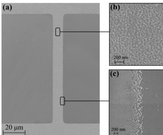
SEM micrographs illustrating the VO<sub>2</sub> micro-bridge, which is also shown in Fig. 1(c). Panels (a), (b), and (c) depict the whole structure, a centrally positioned portion of it and an edge part, respectively.
