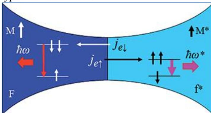
*Schematic of spin-flip photon emission in a spin-majority/minority ferromagnetic point contact, for negative- and positive-bias polarity, carrying predominantly spin-down and spin-down electron currents. The arrows of different colours and thickness illustrate the expected different radiation frequency and intensity in the two cases.*
