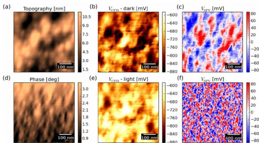
*Example of images obtained by super sensitive Electrostatic Force Microscopy, where different domains are clearly visible with size in the order of 50–100 nm.*
